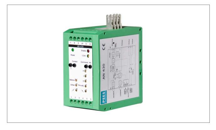
The AN430 controller module has been developed, with the controller and servo amplifier accommodated in a single housing, for actuation of servo valves. The servo valve section can be supplied for four different current ranges ( $\pm 20$ mA,  $\pm 100$ mA,  $\pm 200$ mA,  $\pm 300$ mA). Special types for other valve currents are also possible.
