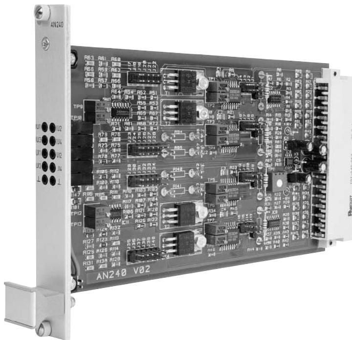
**The AN 240 converter module has been developed to convert current signals to voltages and voltage signals to currents.**
