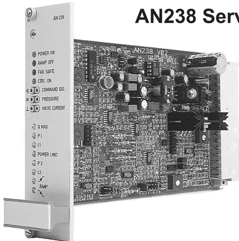
**The AN238 servo amplifier has been designed for the control of axial piston pumps valves in conjunction with servo valves.**
